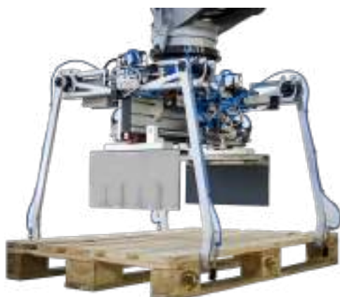
PINZA INTERFALDA/PALLET PALLET/INTERLAYER GRIPPER
